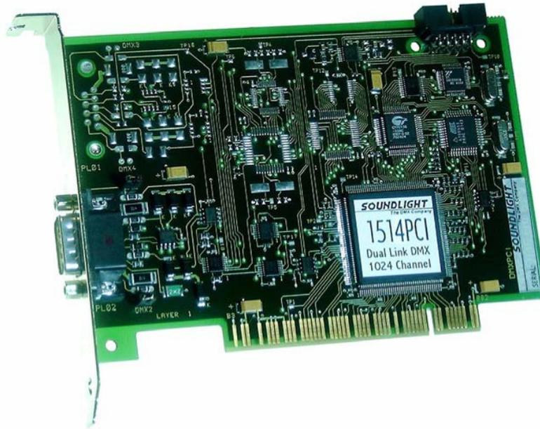
The SoundLight DMX PCI offers up to 1024 DMX input channels or 1024 DMX output channels or combination (512 inputs and 512 outputs). This card handles two complete DMX in/out links in parallel. Up to four cards can be installed in one PC.
