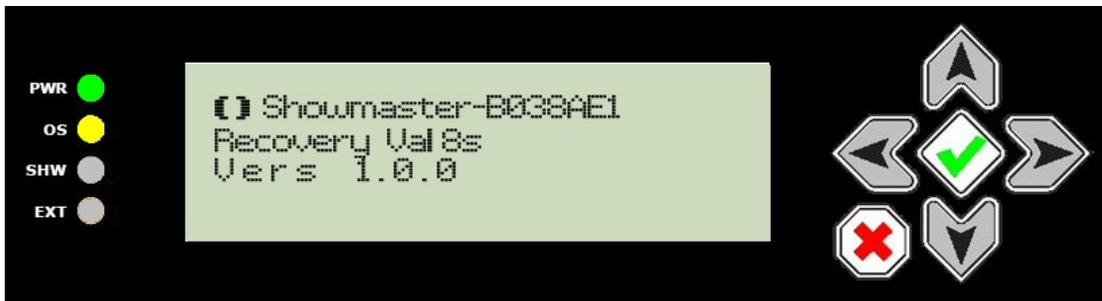
Confirm by pressing the *UP* button a second time to activate the Recovery Mode. The LCD panel displays a Recovery Mode message.
