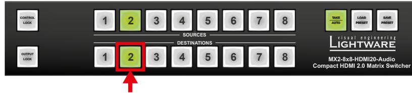
**Step 2.** Press and release the **Output Lock** button; it lights up in red, and lock function is activated at once. No source can be changed at the locked destination.
