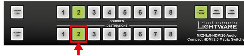
**Step 2.** Press and release the desired **source button**. The switch action will be executed immediately. Switching between sources to the selected destination can be done directly.
