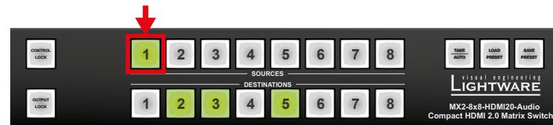
Sample drawing shows that Input 1 is currently connected to the Output 2, 3, and 5 ports.
