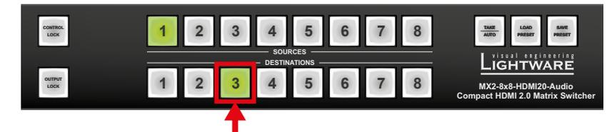
Sample drawing shows that Output 3 is connected to the Input 1.
