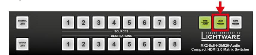
**Step 2.** Press and release the desired **source (memory address) button** (source 1 to 8). Now the selected preset is loaded.
