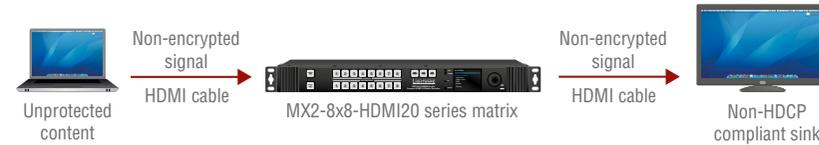
Not-HDCP compliant sink is connected to the matrix. Some sources (e.g. computers) always send HDCP encrypted signals if the receiver device reports HDCP compliancy, however, HDCP encryption is not required all the time (e.g. computer desktop image). If HDCP is enabled in the matrix, the image will not be displayed on the sink.
