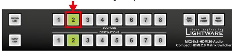
**Step 2.** Press and release the desired **destination buttons** which have to be (dis)connected to/from the selected source. The preselected destination buttons will blink. If no button is pressed for three seconds, the buttons will turn to dark.
