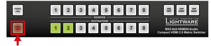
**Step 2.** Press and release a **destination button**; it starts to blink (more destinations can be selected sequentially).
