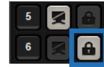
**INFO:** Loading a preset does not change either the lock state or the switch state of a locked output. If an output is locked to an input before preset loading it will also be locked to that input after preset loading, so locked outputs ignore the preset.
