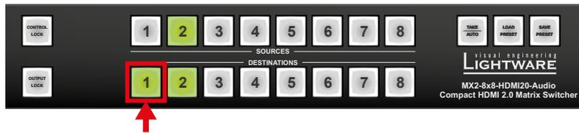
**Step 3.** Press and release **Take** button; the selected input is switched to the selected output(s).
