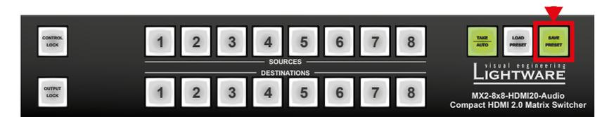
**Step 2.** Press and release the desired **source (memory address) button** (source 1 to 8). Now the current configuration is stored in the selected memory.
