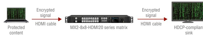
All the devices are HDCP-compliant, no manual setting is required, both protected and unprotected contents are transmitted and displayed on the sink.
