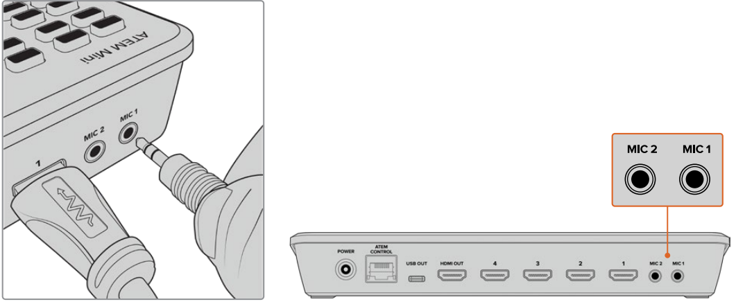
Connect microphones to ATEM Mini's mic inputs
