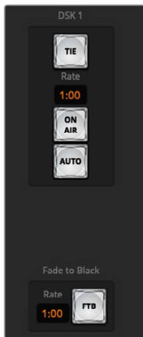
Downstream key and fade to black
